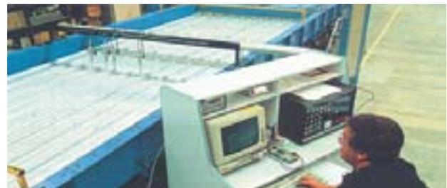
Wind Pressure Testing Rig
